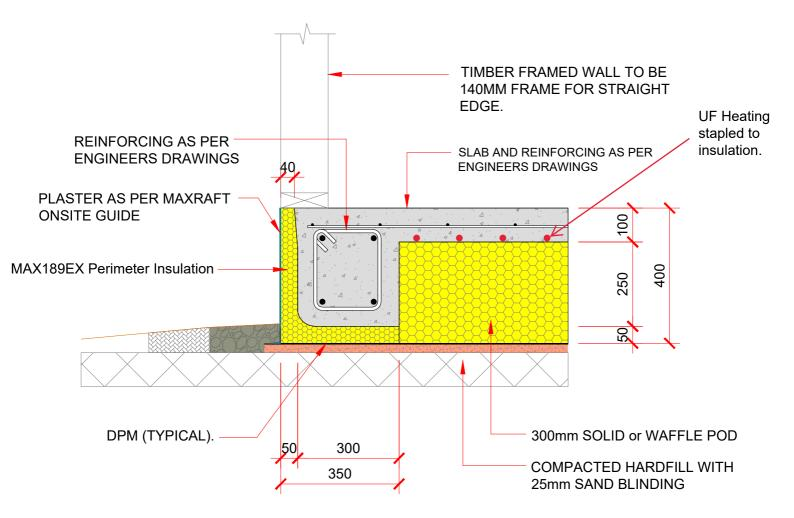
MAXRaft OR MAXRaft Plus+ 400mm Detail
